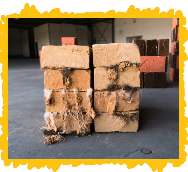
Bricks made with sheared sheep wool!
