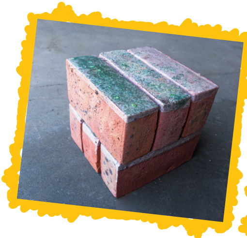
Brick glaze made from crushed glass bottles
